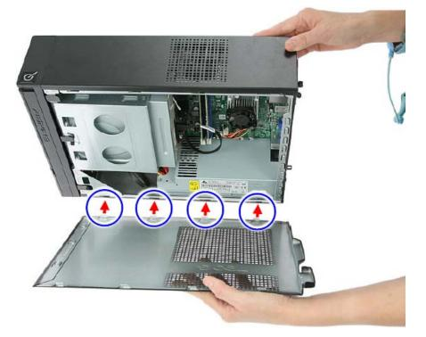
2. Align the tabs on the upper edge of the side panel with the notches on the top side of the chassis.
